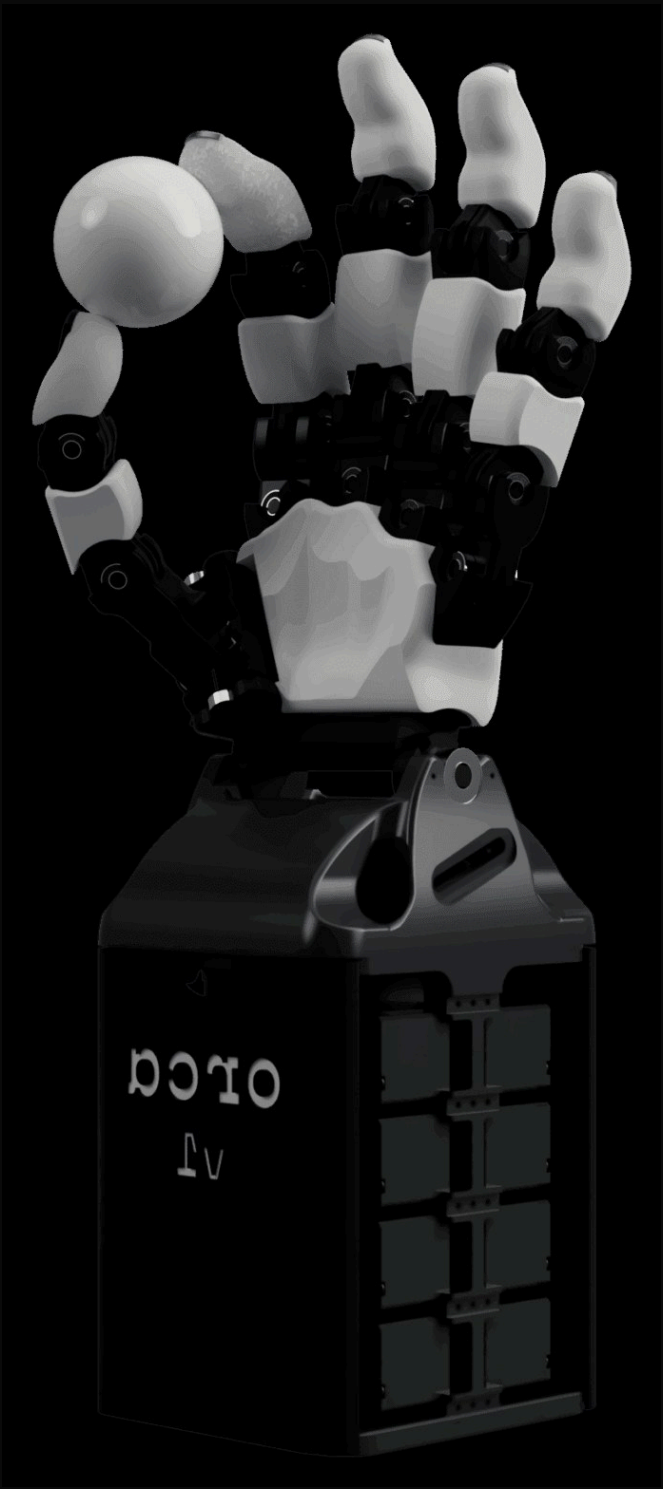
Assembled base configuration. Seventeen degrees of freedom, tendon driven, printed in full.
