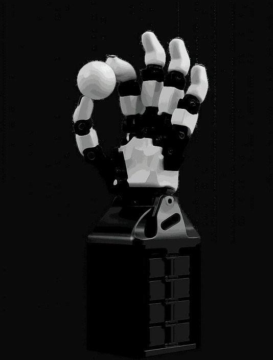
Full hand, printed and assembled, on the actuator base.
